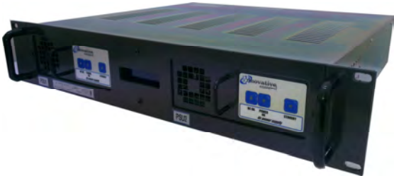
2 x SR250C/i chargers (front removable) in 2U rack
