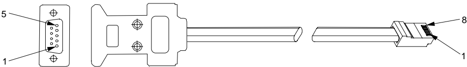
Fig. 5-7: RS485 cable with DB-9 connector.
