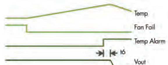
Over-temperature and Fan Fail
