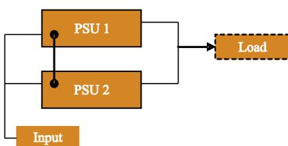
The **second reason** to connect units in parallel, is to provide a back-up should one unit fail. This is also called **N+1 redundancy**. N is the number of units you need to power the load, plus 1 as the back-up. If for example you need to power a load of 600W with redundancy, you could use 2 x 300W + 1 x 300W solution, or 1 x 600W + 1 x 600W.
