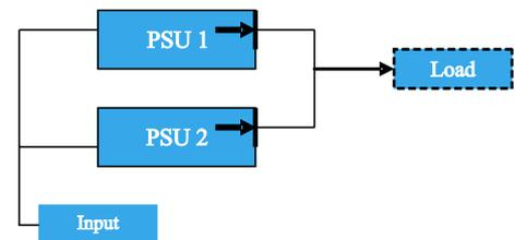
Fig 3 illustrates an N+1 redundant system with the power supplies installed in a 19in rack assembly, fully wired, that allows the modules to be replaced under load conditions. This is referred to as a **Hot-Swap** system. The great benefit of this approach is that replacing a faulty module takes only minutes and there is no need to shut-down the equipment.
