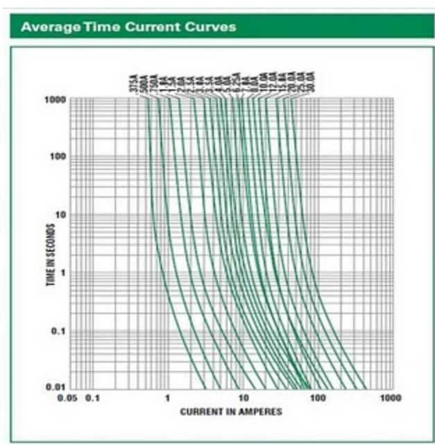
Going back to the power supply evaluation data, one can see that the inrush current is a maximum of 25.65A and that the time for that pulse is say 3ms (worst case). From the above graph, even at 10ms (0.01s) the current would have to be some 70A for the 4A fuse to blow, giving an adequate design margin.
