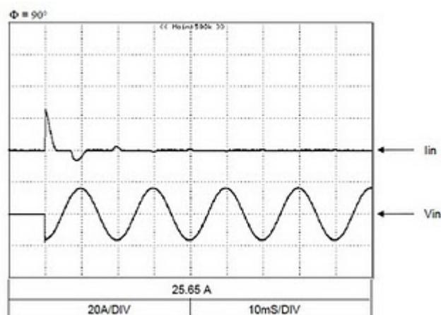
You can see the AC is applied at the peak of the AC input voltage to measure worse case conditions. The peak inrush current is 25.65A for a period of 2-3ms with what we call a cold start, in that the inrush thermistor is initially at room temperature (and in a high resistance state).
